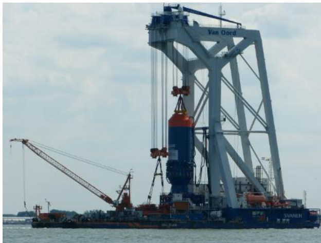
Svanen – 6000 tonne Crane Barge, Holland
