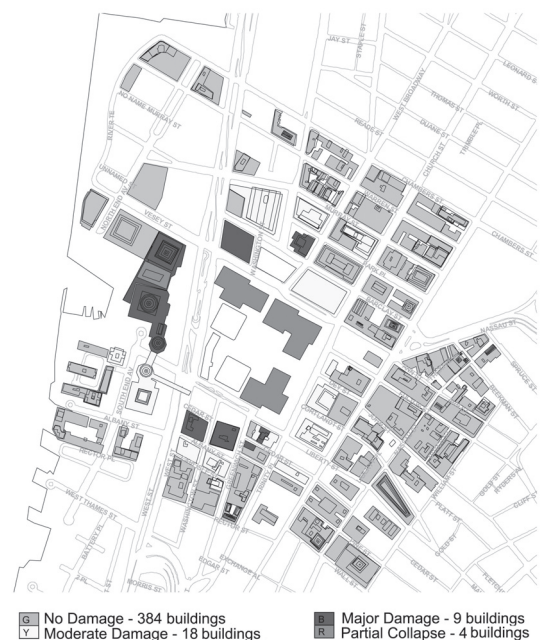
ATC-20 building evaluation results after WTC collapse. Source: New York City DOB/DDC/SEAONY
