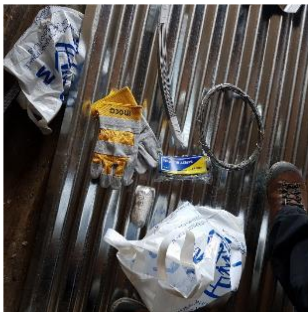
Some of the durable roof-kit components: CGI, tie-wire, packet of nails, safety glasses & gloves
