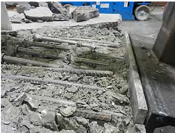
Failed CL-3 Specimen (Note: Rotation of embedded bracket relative to orientation of deck reinforcement)
