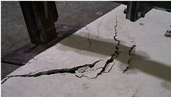
CL-3 Specimen during Testing (Note: Loss of top cover concrete & confinement of embedded bracket)
