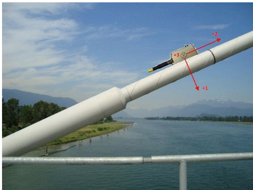
Figure 8 Accelerometer Mounted on Stay Cable of Pitt River Bridge
