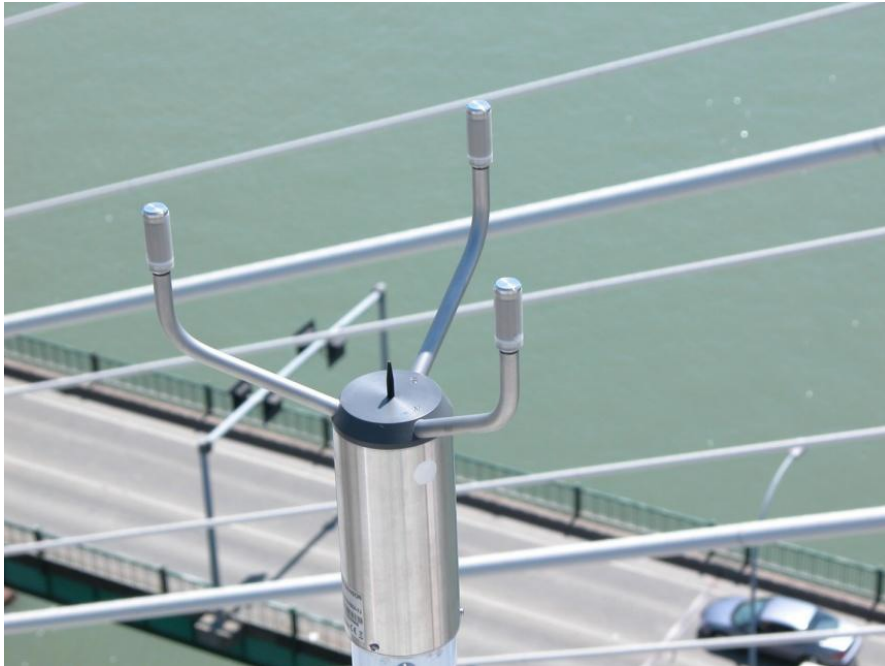
Figure 7 Wind Sensor Mounted on Top of Pylon at Pitt River Bridge
