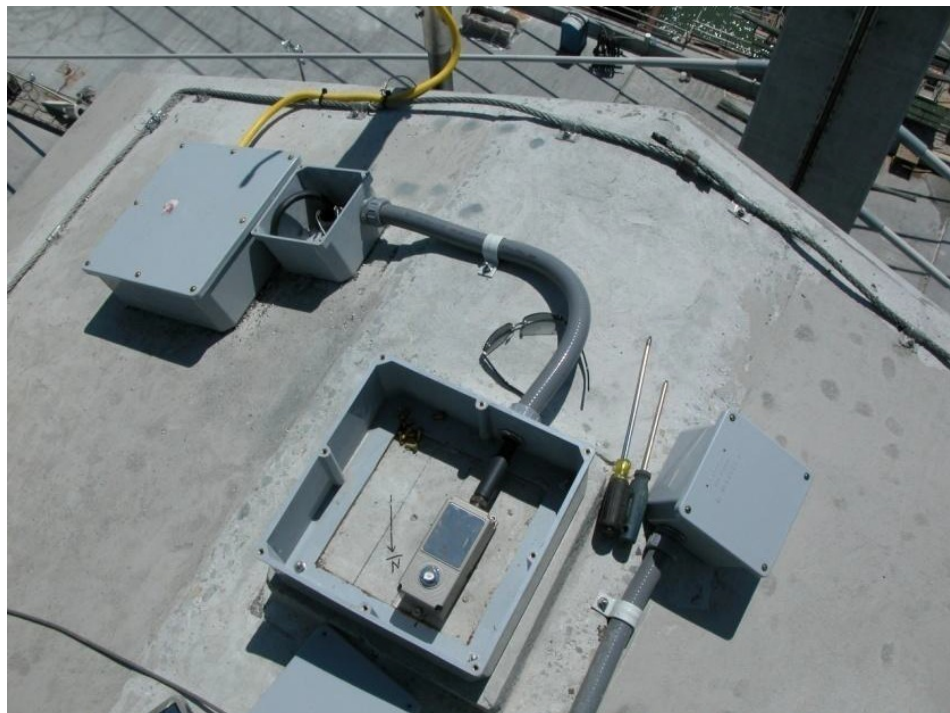
Figure 6 Accelerometer Mounted on Pier of Pitt River Bridge
