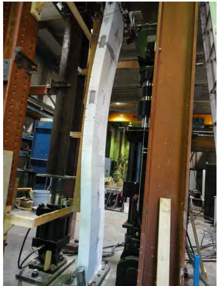
End region buckling behaviour of tall reinforced concrete block masonry walls.
